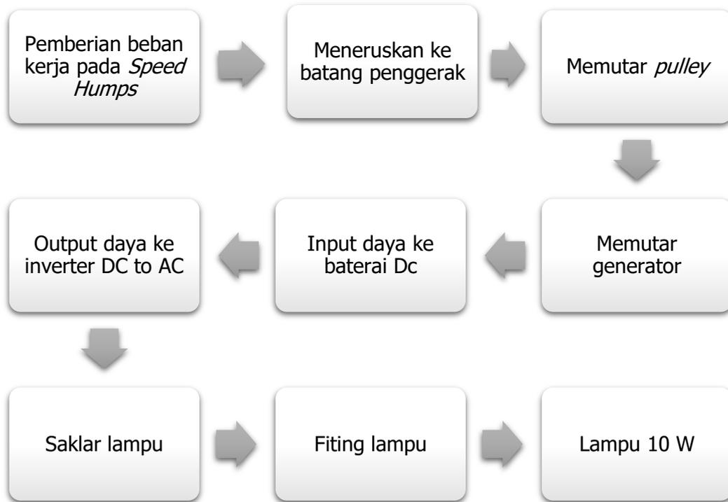
Gambar 2. Diagram kerja *speed humps*
