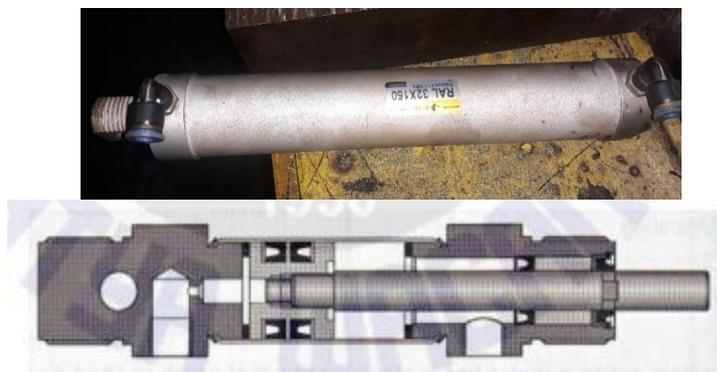
Gambar 7. *double acting cylinder*
