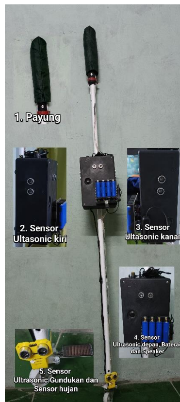
Gambar 6. Hasil perancangan hardware alat
