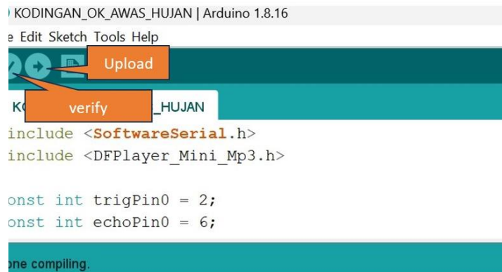
Gambar 5. Proses uploading program ke arduino
