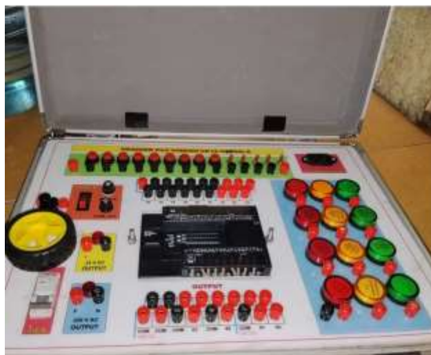
Gambar 6. Hasil trainer PLC Omron CP1E
