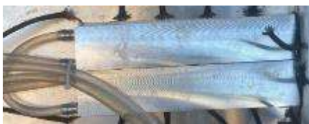
Gambar 11. Sistem pendingin waterblock
