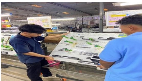
Gambar 7: Penanganan Jig Board
